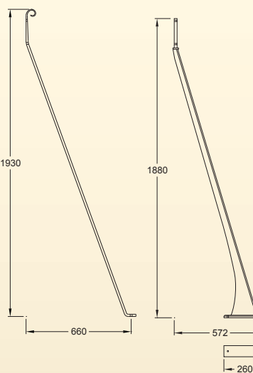
GA109 Wrought railing stay. For use with all railing panels except Stirling full height
